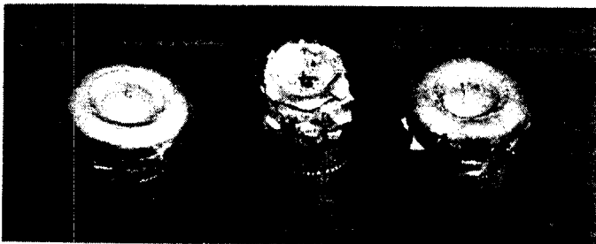
Shown are Winchester 85-gr. Silvertips fired from a 380 Auto. The bullets on either side were fired into thoroughly soaked phone book pages. The bullet in the middle was fired into identical material which had not yet become completely soaked. The importance of using 100% saturated phone books is clear.
